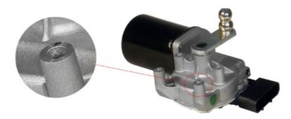
This particularity is due to an agreement between Vehicle manufacturer and Wiper System manufacturer, which permits to obtain a better adhesion between the wiper motor bracket and vehicle body while reducing the risks of self-loosening during operating in a continuous vibrations environment.
