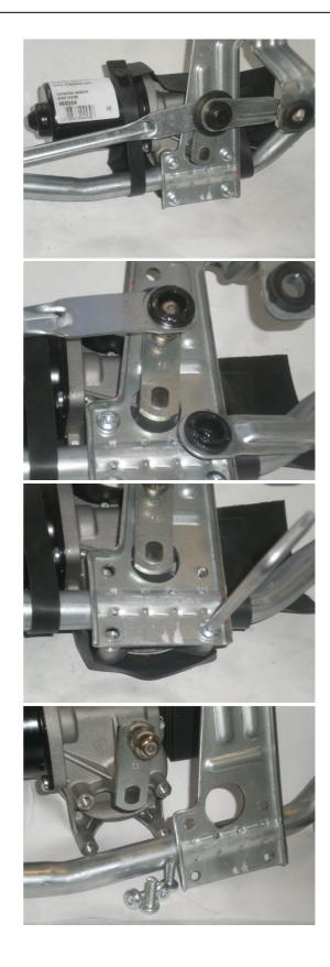
In circled imagine is visible one of the new wiper motor OE fitting holes, without thread. The motor mounting holes have no thread because the fixing bolts are self-tapping.
