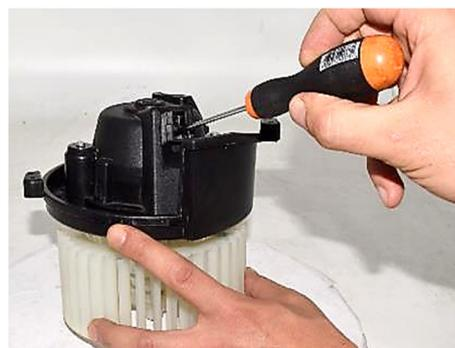
2) Dismantling of connectors compartment (highlighted in green)
