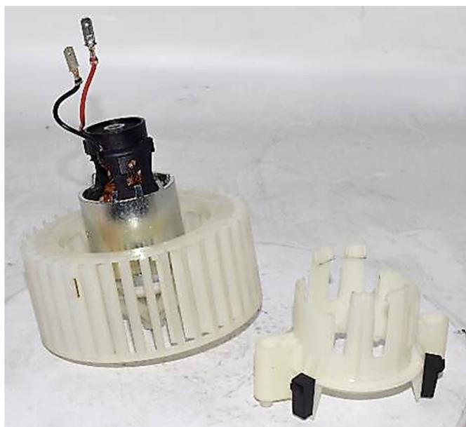
8) Use new interior blower (ERA 664089) and put together each parts, following the reverse process.
