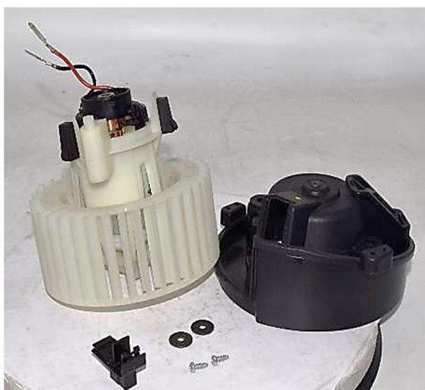
6) Unlocking of the 4 anchor points in interior blower
